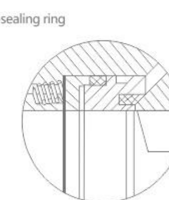
阀座耐火结构 Refractory structure of valve seat
